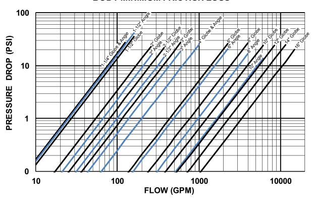
Note: If the valve is to be used for continuous flow, it is very important to maintain a flow rate through the valve below the maximum continuous flow rate. It may be necessary to install a gate or butterfly valve downstream to throttle the flow rate and prevent damage to the valve.
