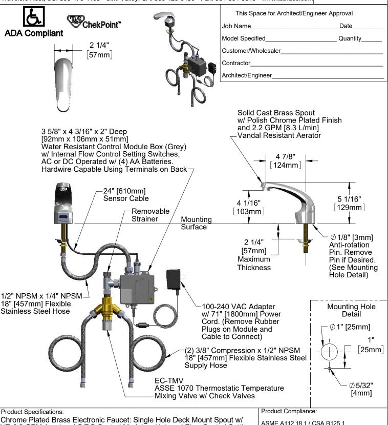
Chrome Plated Brass Electronic Faucet: Single Hole Deck Mount Spout w/ VR 2.2 GPM Aerator, AC/DC Control Module w/ Internal Flow Control Setting Switches, Thermostatic Temperature Control Mixing Valve w/ Check Valves, 18" Hot & Cold Supply Stop Flexible Connector Hoses
