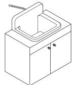
Set the sink at the desired place and mark a horizontal leveled line at where the top of the backsplash will be situated, remove the sink, measure 4-5/16" down from the previous line and mark another horizontal leveled line.
