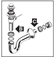
Secure lavatory on hanger as shown in 5. Insert and tighten anchor screws if applicable. Connect hot and cold supply lines to the shut-off valves. Tighten trap joints for watertight assembly. Apply a bead of caulk around the edge which contacts the wall as shown.
