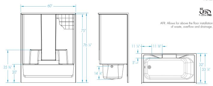
FEATURES Ibs Dimensional Tolerance ± 3%". Dimensions needed for site preparation should be measured from the unit. Aquatic assumes no responsibility for preparatory work.
